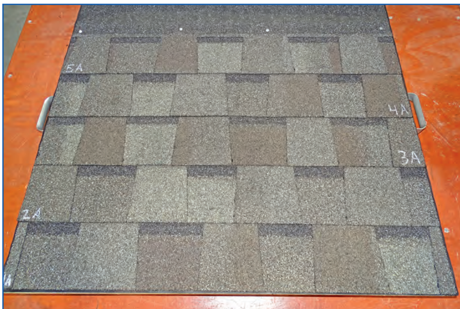
Figure 4 – Laminated shingle test panel.
