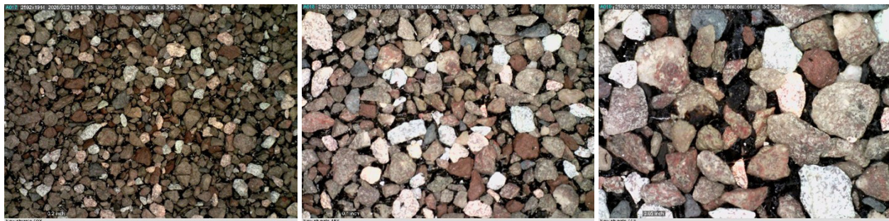
Figure 1: Surface of a new asphalt shingle under magnification. 10X (left), 18X (center), 40X (right)
