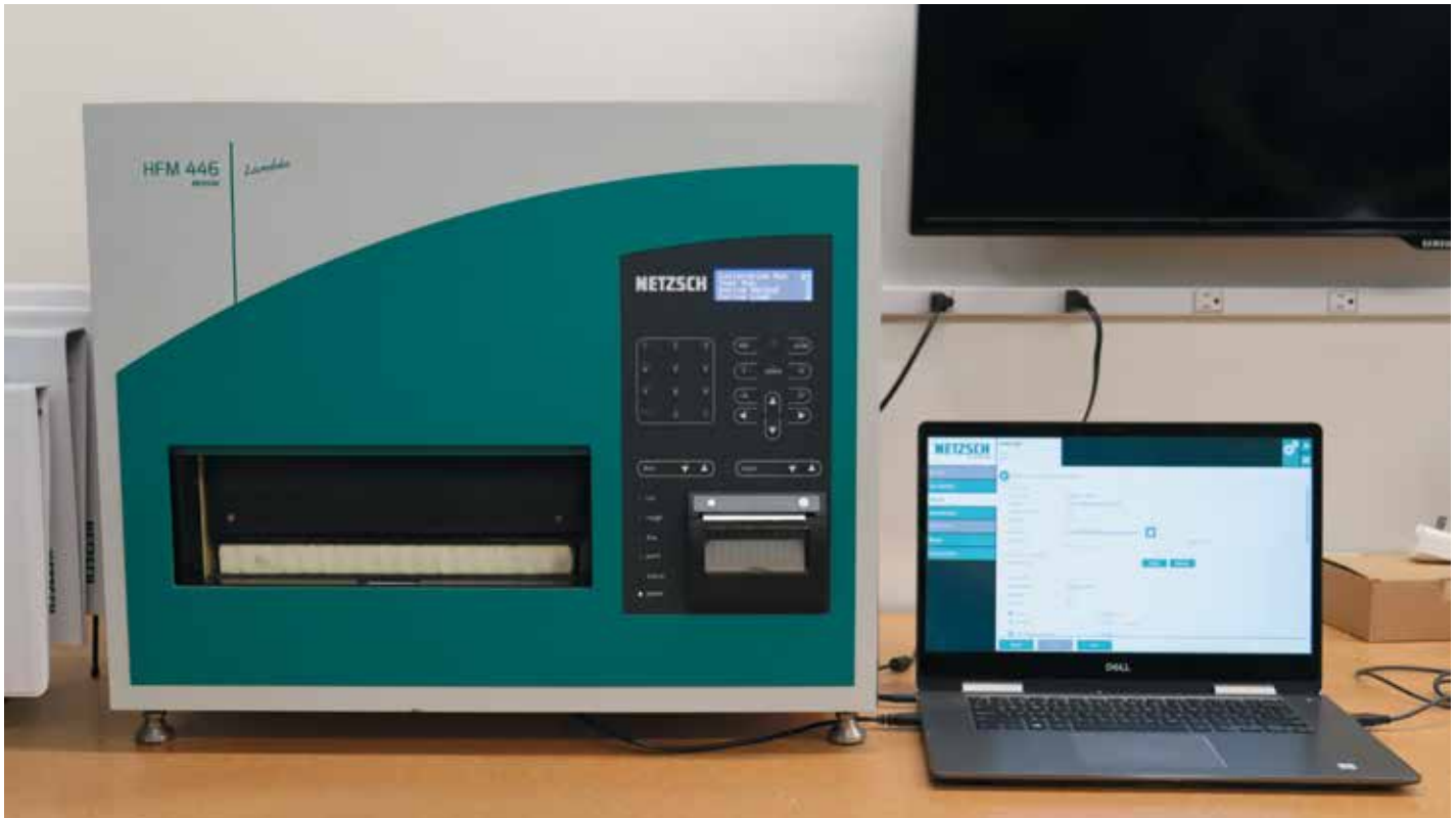
Figure 1. Heat flow meter test setup.
