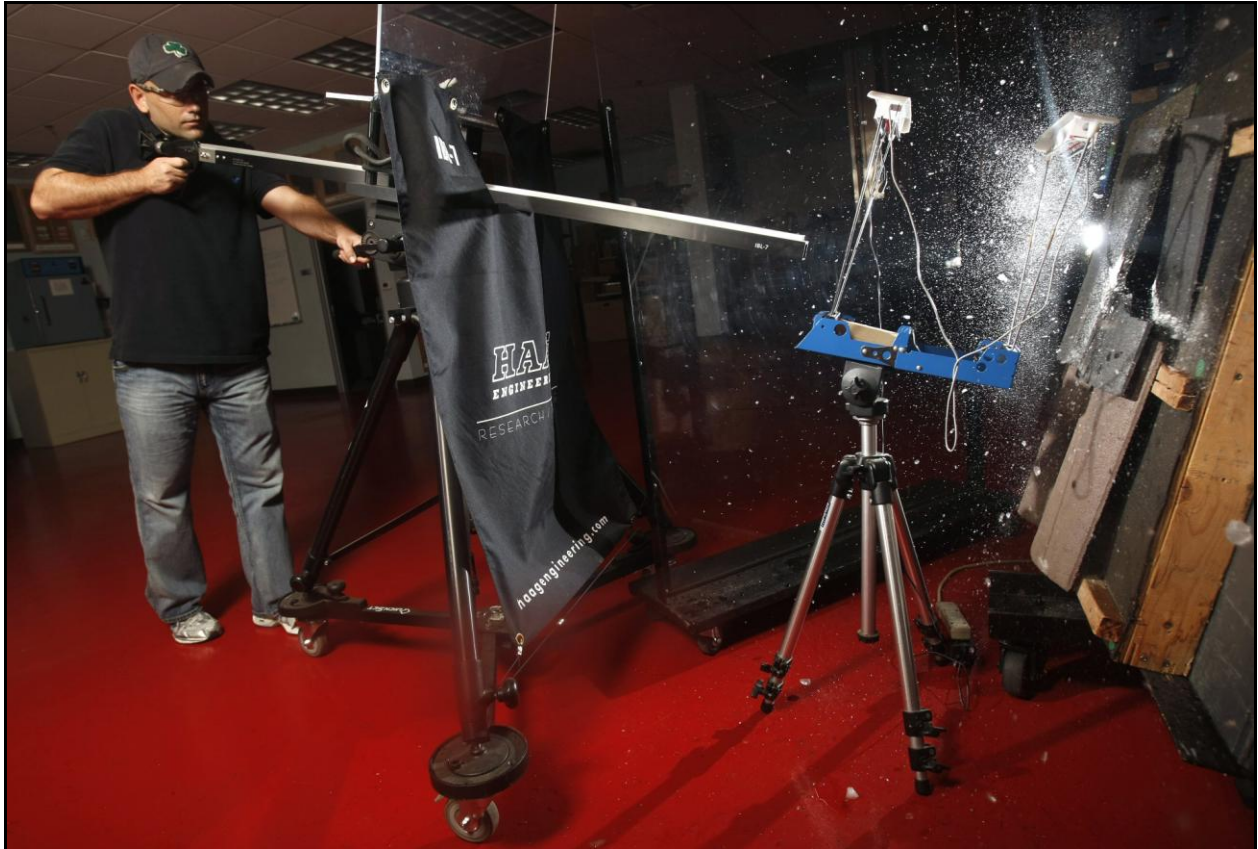
Figure 5. Seventh generation ice ball launcher (IBL-7) with light emitting diode (LED) sensors (chronograph) developed for impact testing.
