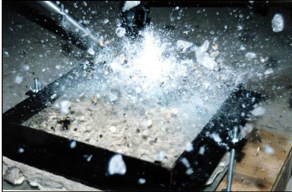
Figure 4. Ice ball breaks apart upon impact removing some of the surface gravel and flood coat on a built-up roof. No damage was done to the underlying roofing plies.
