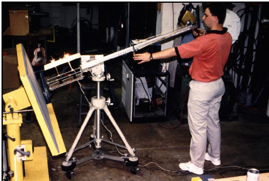
Figure 2. Third generation ice ball launcher (IBL-3) constructed by Haag Engineering Co. for their 1983 impact study. A chronograph was mounted to the end of the launcher to measure the velocities of the ice balls.
