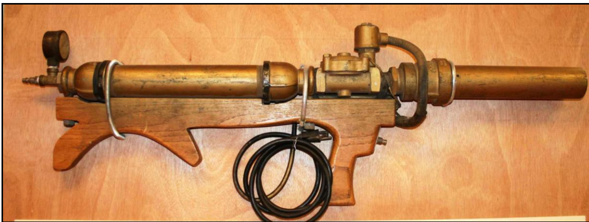
Figure 1. First ice ball launcher (IBL-1) constructed by Haag Engineering Co. in 1963 for their impact study on cedar shingles.
