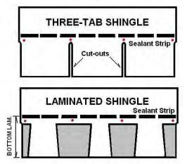
**Figure 5.** The two most common types of asphalt shingles are the three-tab and the laminated. At least four fasteners must be installed per shingle (standard application) as noted by locations of the red dots.
