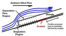
**Figure 3.** Idealized wind flow (blue lines) and resultant positive (plus signs) and negative pressures (minus signs) at the bottom edge of a shingle. From Peterka et al. (1997).
