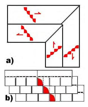
**Figure 15.** Diagonal pattern of shingle overlaps not bonded to the roof: a) roof plan showing open laps (arrows) pointing in different directions, and b) idealized diagram showing red shaded region where tabs could be lifted unimpeded by hand. This pattern extends diagonally upslope depending on the manner in which these shingles were installed.
