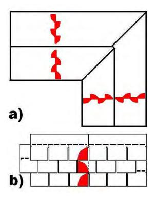
**Figure 17.** Straight-up pattern of shingle overlaps that are not bonded to the roof: a) roof plan showing alternating overlaps not bonded to the roof on each directional slope, and b) idealized diagram showing red shaded region where tabs were not bonded to the underlying shingles. This pattern extends vertically upslope in the manner in which these shingles were installed.
