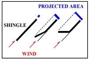
**Figure 4.** Idealized diagram showing the increase in the projected area (blue line) as the shingle is uplifted in the wind.
