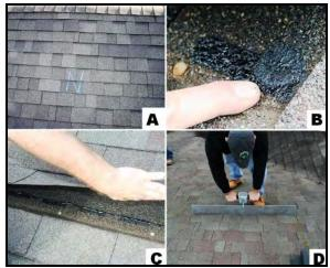
**Figure 20.** Pull tests on laminated asphalt shingles: a) undamaged shingles, b) dollop of asphalt plastic cement applied under shingle, c) bead of asphalt plastic cement applied under shingle, and d) pull test after 30 days.
