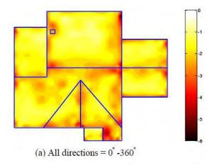
**Figure 1.** Peak negative uplift pressure coefficients  $(C_p)$  on a gable roof from a wind tunnel model. Wind directions were at 10 degree increments. From Liu et al. (2006)
